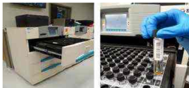
Figure 2: The BACTEC™ MGIT™ 960 instrument and culture tubes used to isolate and identify mycobacterial growth.
